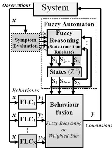
Fig. 3. The proposed behavior-based control structure [16]
